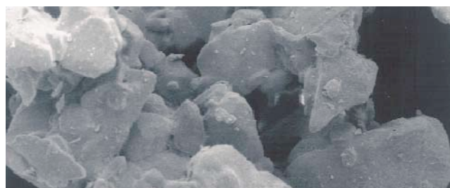
Instant Sugar particle enlarged 600 times. The picture shows the porosity of the particle.
