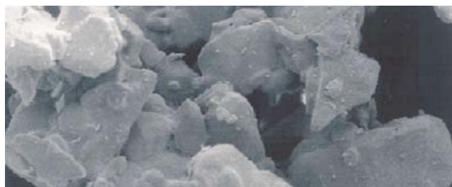
Pharma Instant Sugar enlarged 600 times. The picture shows the porosity of the particle.
